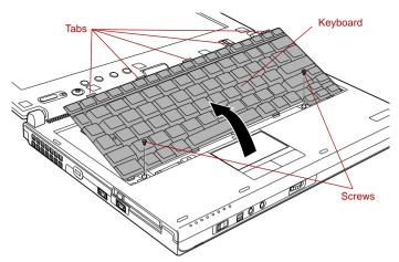
Figure 3-13 Replace the keyboard
